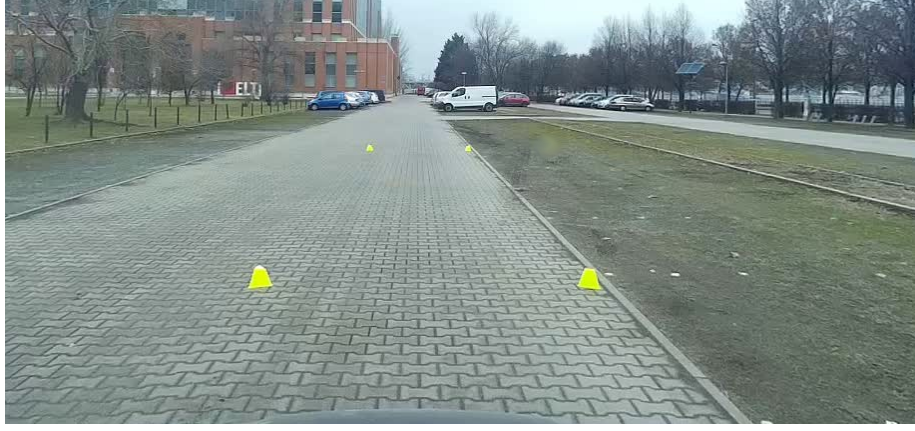
Fig. 3: Four yellow markers are placed in order to estimate the homography. Best viewed in color.
