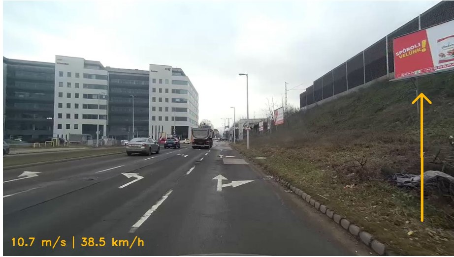
Fig. 6: Estimated speed (bottom left) and vehicle velocity vector (right) are visualized.
