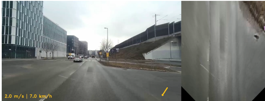
(b) Wrong velocity vectors is estimated when not enough corners are detected due to lack of street lines.
