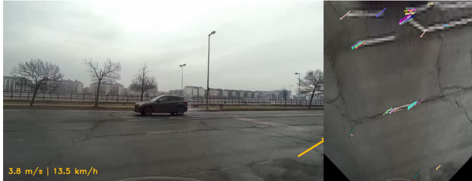
(a) The velocity vector is estimated while the vehicle is turning right.
