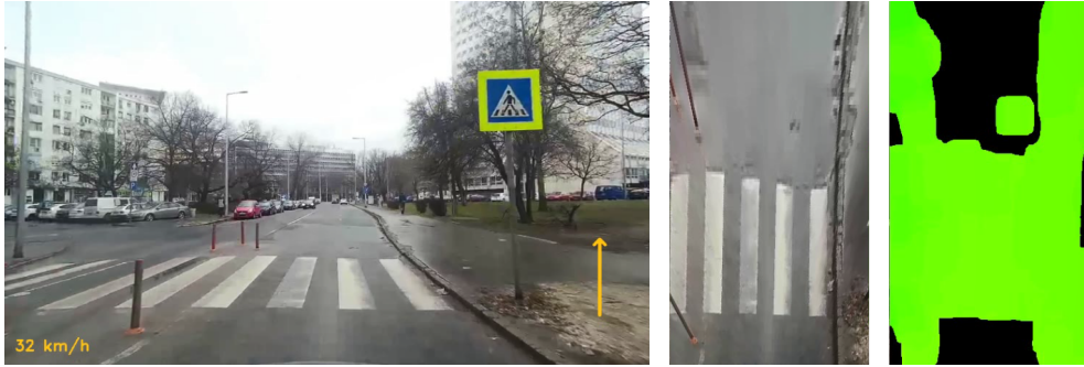
Fig. 7: Left. Perspective image with estimated speed (bottom left) and vehicle velocity vector (right) are visualized. Mid. Top-down (BEV) image. Right. Top-down image motion with heat map.
